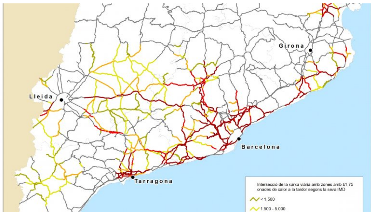
Road network located in areas within more than 20 hot days per year, according to the projections of the SMC in the period 2021-2050 © Source: authors
